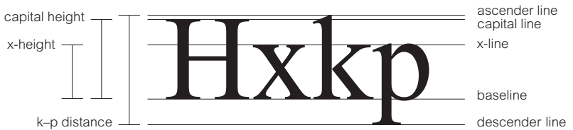
4.4 Typefaces have different proportions; some may have large x-heights and therefore relatively short ascenders, as in the above example, which shows Times New Roman.
